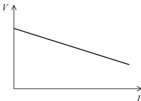
Select the row of the table that correctly identifies how  $\mathcal{E}$  and  $r$  are determined from the graph.
