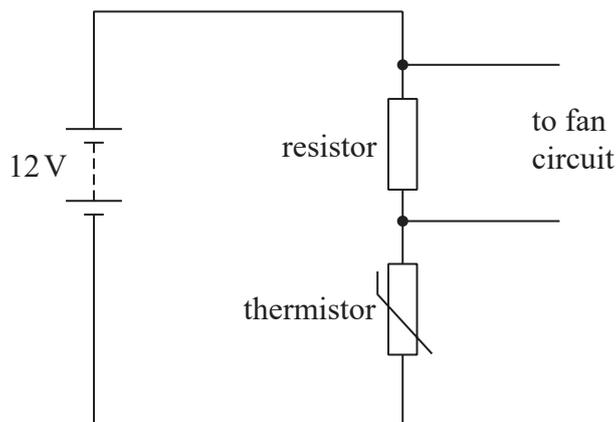
Calculate the resistance of the resistor.
